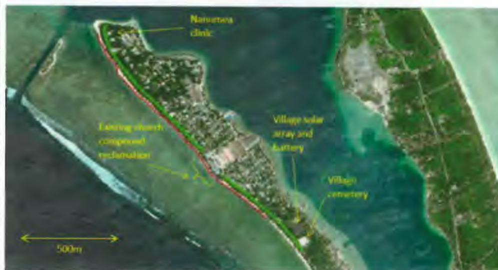
Figure 6. The revised TCAP proposal will protect a comparative 1,500m of shoreline with a mixture of BTB (green line) and a hard revetment at the main church compound (central area where there is a 150m gap in the BTB's). The red line is the original TCAP area of "high value coast" of which the central area of approximately 760m was originally targeted for geotextile bag revetments. Thus, the revised proposal provides protection for an additional 740m of shoreline ensuring important community sites such as the village solar array and battery and main cemetery are also protected from marine flooding during overtopping events.
