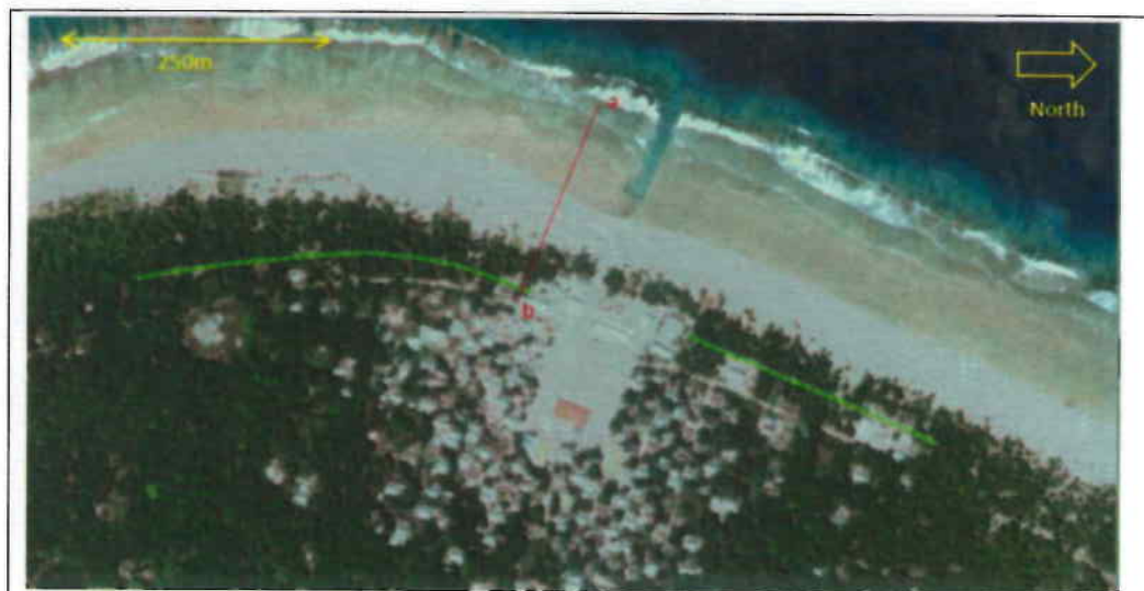
Figure 4. Close up of Nanumaga Village area showing location of planned BTB. The location of the BTB is aligned to the crest of the natural storm berm system and is some 7m above the reef platform (which in turn approximates mean sea level). Note that most of the buildings (other than the church and new clinic buildings) are built on the landward side of the main road likely because of the known impacts of storm waves. This means the BTBs do not interfere with or interact with the built environment for most of their length. Their foot-print mainly lays in open coconut woodland. Details of transect a / b appears below.
